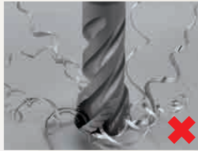
Thread chips can cause tool breakage
